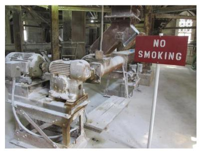
Figure 3-35: Lime Screw Conveyor
